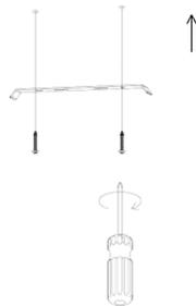
Fix bracket with screw into the ceiling
